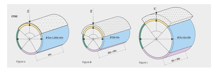
Under the same production levels, the geometry of Marzoli C702 Card allows to reduce the density of the processed material in the carding area with mobile flats (See *Figure a*). This entails a thinner layer (Ha) of the carded material with two positive effects:
