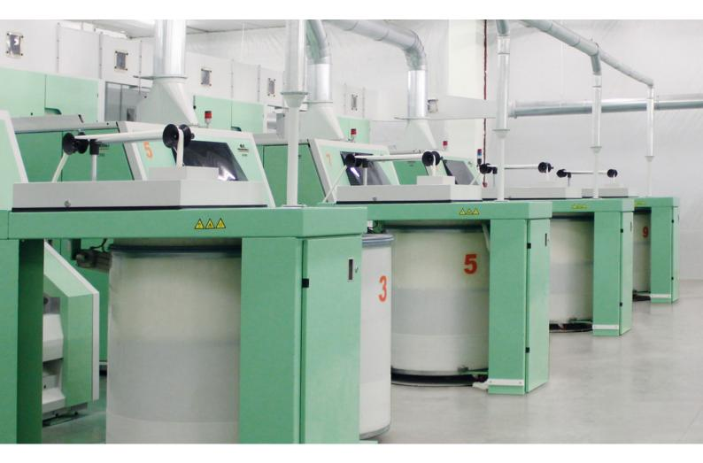
Carding has always been and will continue to be one of the most important phases of the spinning process. Only with an effective carding of the fiber the spinner can produce a homogeneous, regular, resistant and clean yarn and therefore ensure efficiency and quality in all downstream operations.
