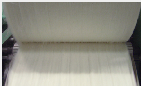
LW3: regularity of the superimposed cotton layers for a superior quality of the laps
