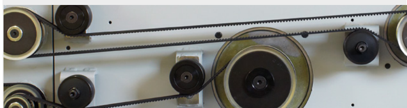
Simple and reliable Toothed Belts Drive System.
