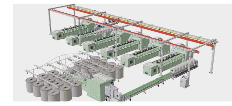
The new fully automatic lap transport system, totally manufactured by Marzoli, guarantees the simultaneous transport of laps from the LW3 lap winder to the comber.
