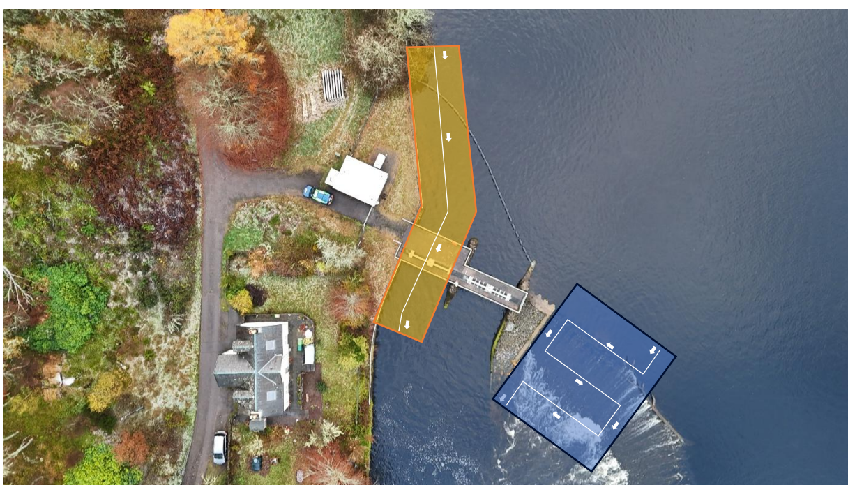
Figure 5-1. Indicative overview of two potential locations for the vertical slot fish pass; comprising either the bankside bay of the existing SSE sluice gates (orange) or the most upstream section of the service weir (blue). White lines and arrows denote the centreline of the potential flow route and requirement for changes in direction ( not to scale ).
