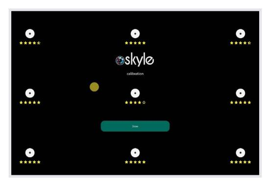
In the App Settings you can switch the standard calibration method between a 1-, 2-, 5- and 9-point calibration.
