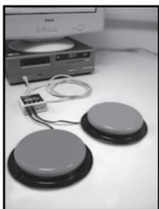
To use a switch with **Switch Skills 3**, you will need to attach it to the computer using an interface box. There are a number of interface boxes available. The **Inclusive Simple Switch Box** is inexpensive and easy to use.
