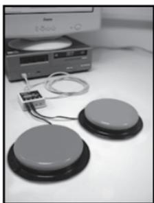
To use a switch with **Switch Skills 3**, you will need to attach it to the computer using an interface box. There are a number of interface boxes available. The **Inclusive Simple Switch Box** is inexpensive and easy to use.
