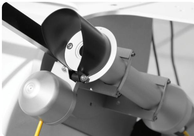
Kipp & Zonen smart radiometers are individually addressable and can be linked together in a multi-drop configuration to a single RS-485 cable that can be hundreds of metres in length. This makes installation easier and saves on cable costs. The SHP 1 can be mounted on a Kipp & Zonen sun tracker and linked to smart pyranometers and pyrgeometers to make a complete digital solar monitoring station.
