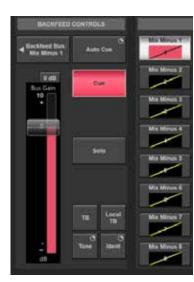
A Backfeed feature with mix minus assignment places the controls of a Mix Minus return bus directly on the incoming outside source channel. This greatly simplifies operation for complex external line control, without the need to navigate to other layers or other systems.
