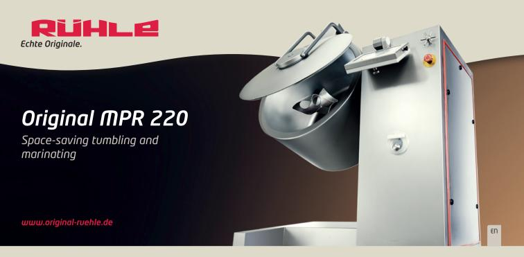
With a footprint the size of a Euro palette, the Original MPR 220 has a container volume of 220 lt and can hold about 160 kg of meat. It is perfectly equipped for tasks from cooling to vacuum treatment to variable arm speeds for achieving perfect results.
