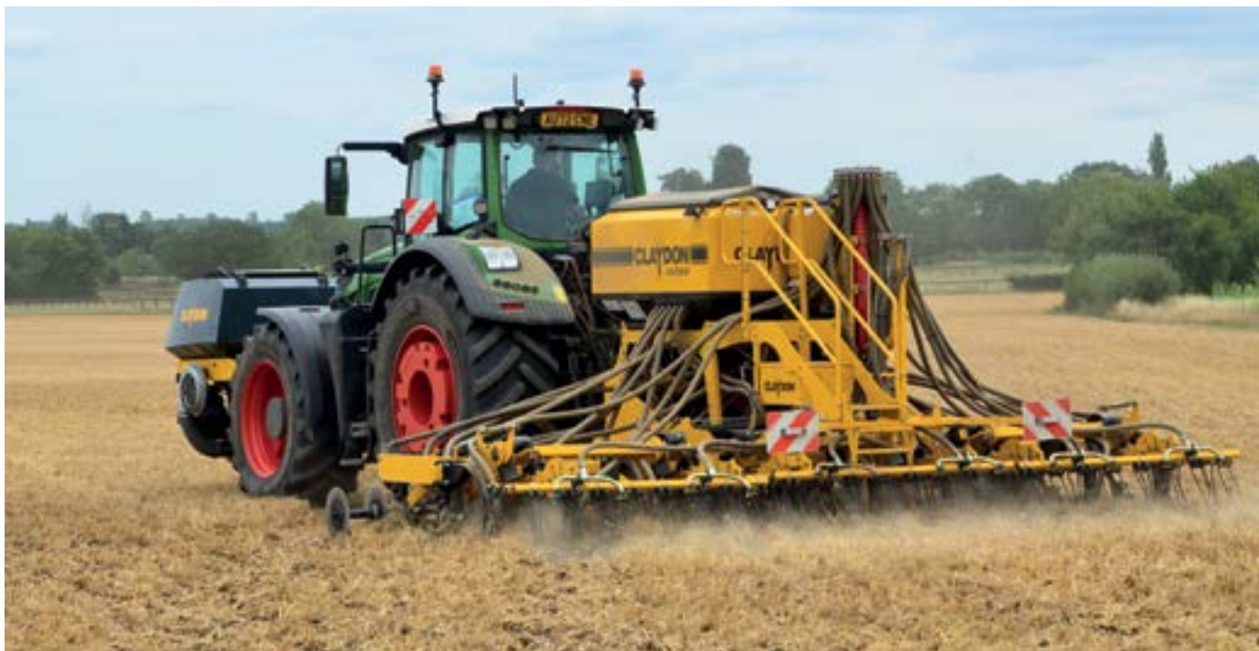
The Claydon farm's 6m Evolution one-pass drill and double front hopper combination establishing a cover crop.
