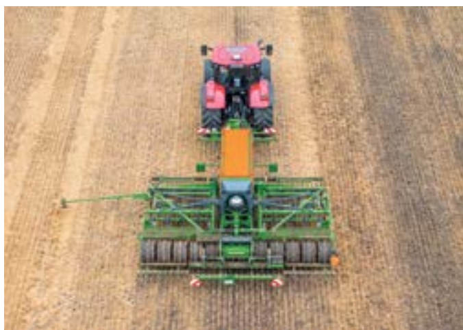
The Cayena 6001-C working in stubble, with the rear Matrix tyre packer reconsolidating only the seed rows after placement
