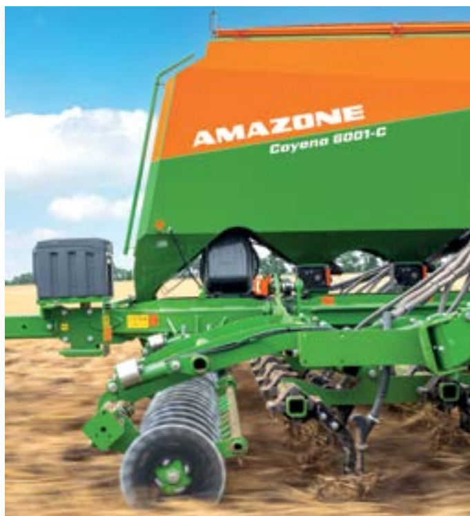
Optional cutting discs ahead of the Cayena's tine coulters help manage surface residue and improve passage through the drill
