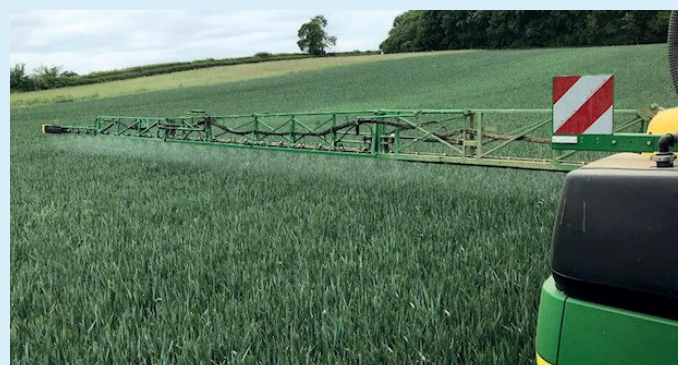
Twin select applying 200 litres per ha via 035 and 025 guardian air nozzles together
