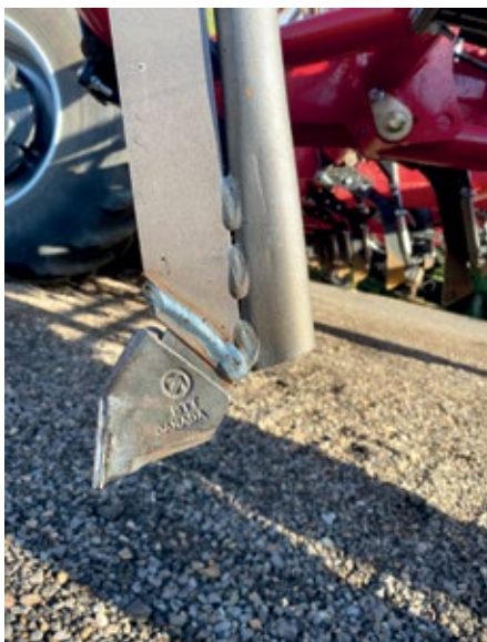
First Trial Coultter Tip Tine, VOS 19mm Tip with fixed seed tube like the Amozone Cayenna.
