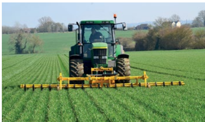
The Claydon TerraBlade did a really good job of removing blackgrass
