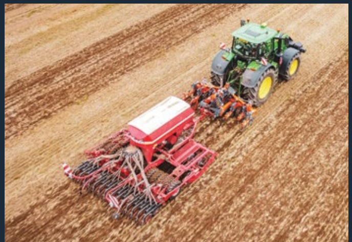
Toolbar when fitted with optional rear hydraulic linkage/towbar to pull secondary cultivation equipment or drill
