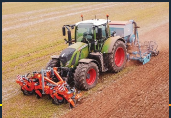
Front mounted 4m running with combi drill
