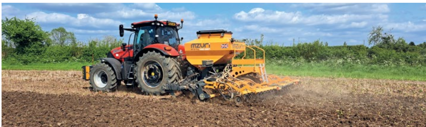
The Pro-Til iGen features independent coulters each with its own depth wheel for accurate seed depth control.
