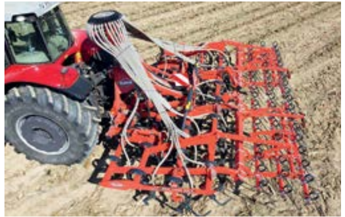
KUHN's Prolander is now available with a distribution head and TF1512 front tank to enable the cultivator to plant crops and cover crops and apply fertiliser.
