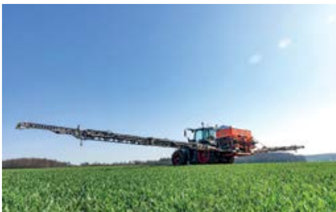
The KUHN Aero 32.1 features a 24 nozzle boom and can be specified with a 3200 litre hopper.
