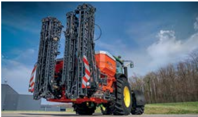
The mounted KUHN Aero 32.1 is available in 27, 28 and 30 metre working widths, but folds to a compact load on the rear of the tractor.
