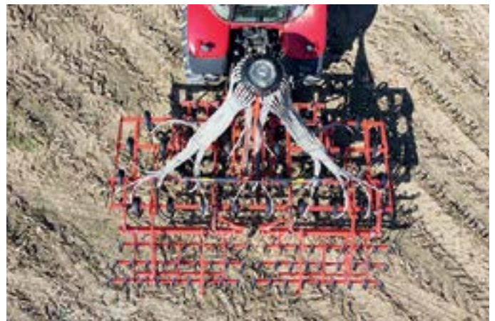
The distribution unit can be controlled with KUHN's ISOBUS CCI terminal or a tractor ISOBUS terminal.
