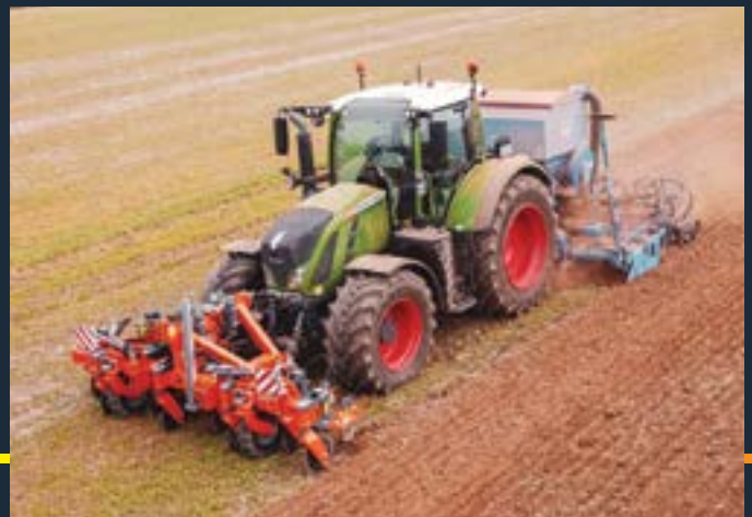
Front mounted 4m running with combi drill
