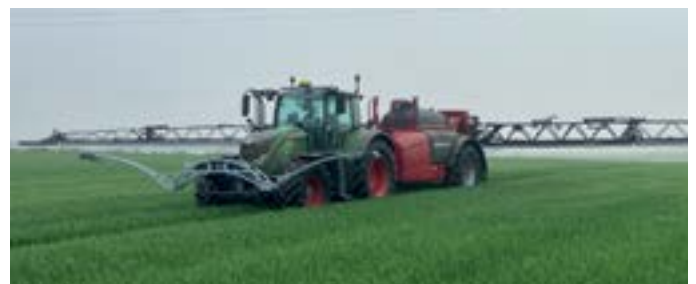
Input use efficiency is key – An NIR sensor is used to variably apply crop inputs, aided by GPS technology to control the sprayer on a crop of spring oats. This has taken a bit of adaptation as the algorithm is designed for wheat.
