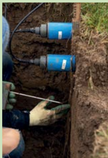
Sensors to monitor the pH, electrical conductivity, soil temperature and soil moisture all of which will demonstrate that weathering is taking place
