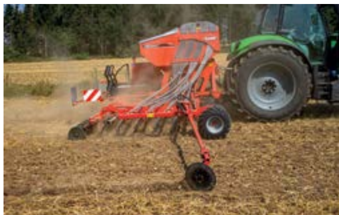
The KUHN Megant 602R can be specified with an additional tank to sow multiple products in one pass.
