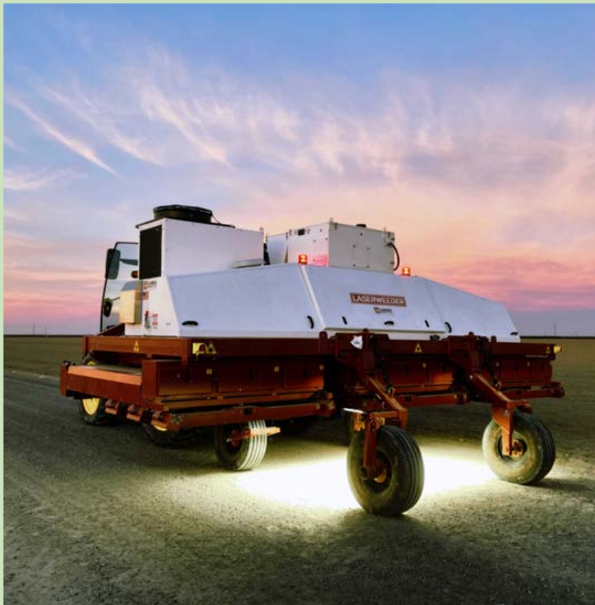
The Carbon Robotics LaserWeeder features 30 industrial carbon dioxide lasers and has a claimed output of about 0.8ha per hour.
