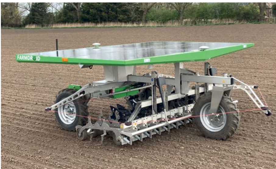
Imported into the UK by Opico, the FarmDroid FD20 uses solar power stored in batteries as its sole source of energy.
