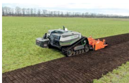
ASC Autonomy suggests two or three AgXeed tracked tractors could replace one large conventional tracklayer.
