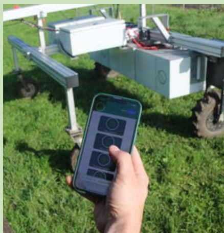
The rover can scout for the crop, the weeds or both, and have the data available on a laptop, tablet or phone for decision making in real time.
