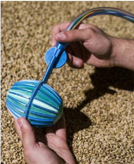
The Cover is a sensor that burrows through a heap of grain gathering data on quality and condition.
