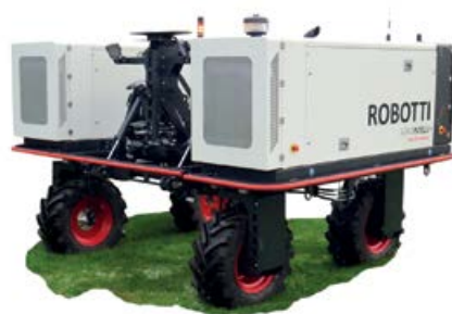
The new version of the Agrointelli Robotti requires only a single engine, thanks primarily to hydraulic system upgrades.
