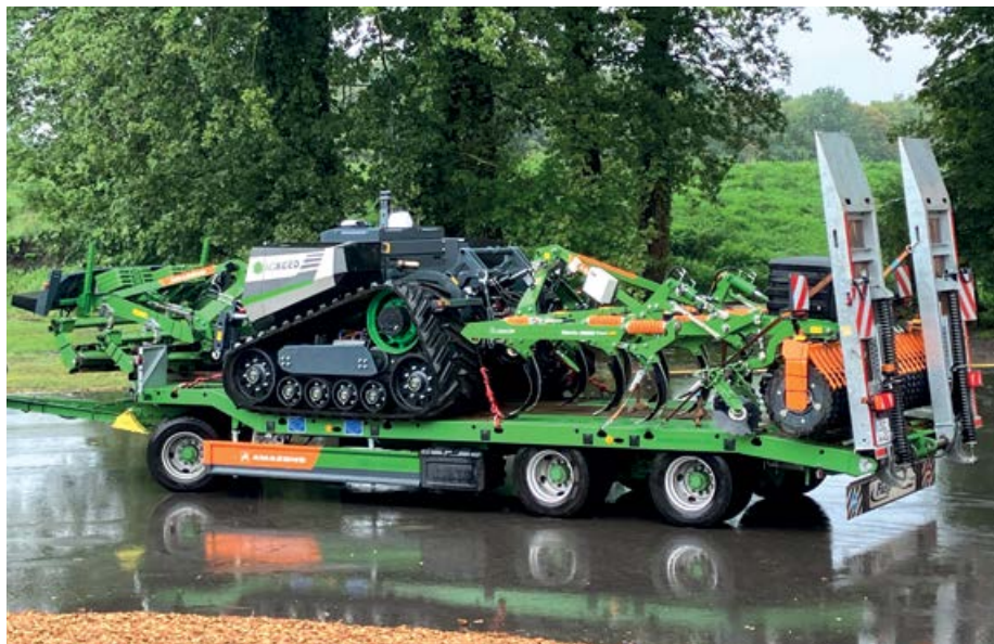
AgXeed offers three- and four-wheeled autonomous tractors, but promotes this 156hp tracked version as its primary arable offering.
