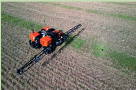
SRC's Tom scouting robot is now on version 4, with a more rigid boom, an upgrade to its eight cameras and a modular design.
