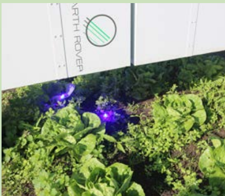
CLAWS uses semiconductor LEDs to generate light that is then concentrated precisely onto the meristem of a weed seedling.
