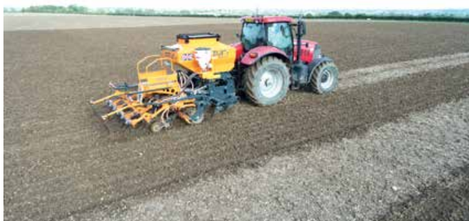
The Pro-Til iGen 300 fitted with independent spring loaded coulters with individual depth wheels
