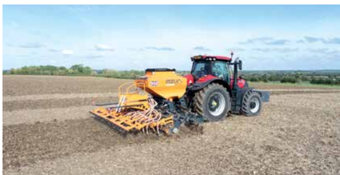
The Pro-Til iGen 480 fitted with Twin Spring Tine Coulters
