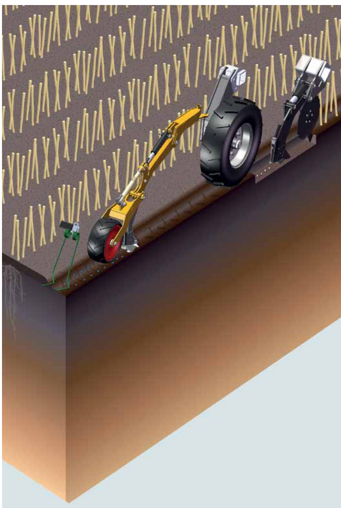
Mzuri leg configuration and coulters- demonstrating fertiliser placement, reconsolidation and seeding
