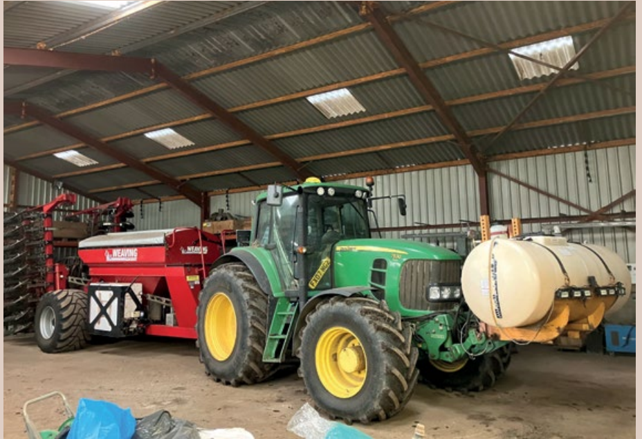
The GD drill ready to go with front and side tanks for liquid fertiliser amendments
