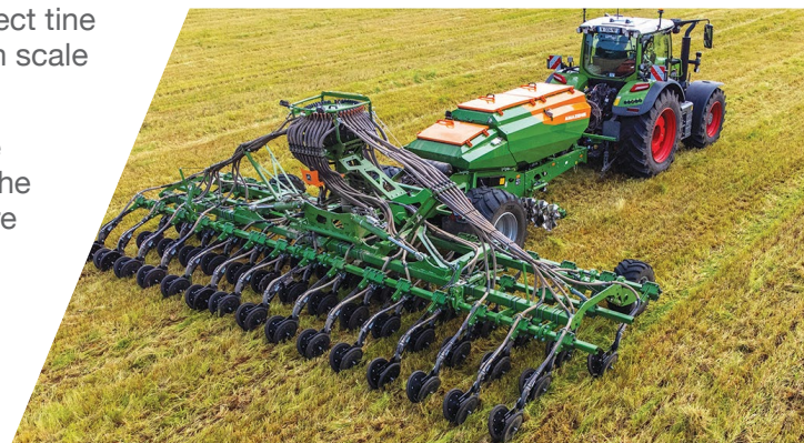
The NEW Condor range - in working widths of 8 and 9 metre. Triple hopper size 4,100 litres (50% | 30% | 20%)
