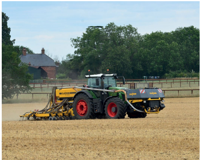
Drilling a cover crop immediately behind the combine, after the Straw Harrow had been used to evenly distribute the chopped straw.
