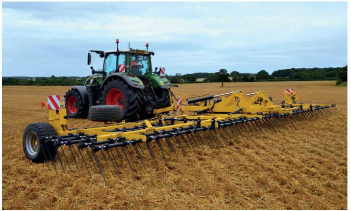
This 15m Claydon Straw Harrow is at the heart of the farm's stubble management approach.
