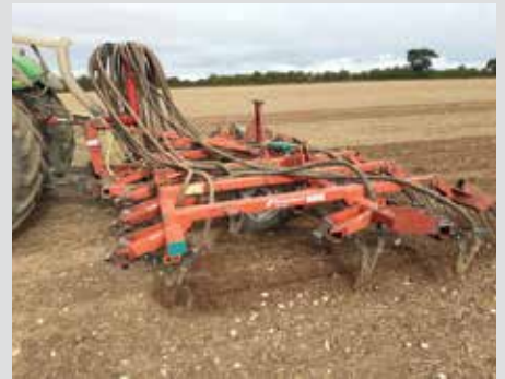
Cultivator conversion with Metcalfe legs
