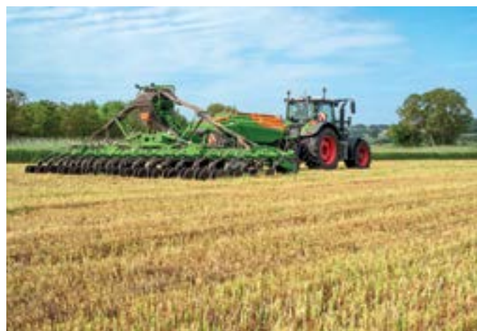
The Condor 9002-2TC working in stubble, with its individually guided coulters following the soil surface
