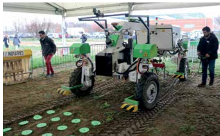
The Orio is a seeding, weeding 100% electric autonomous tool carrier.
