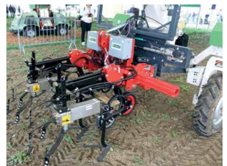
K.U.L.T. Kress' InRow eActuators work in between plants within the row to hoe the soil as close to the crop as possible.
