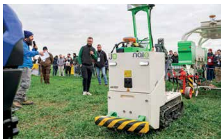
Just 1m wide, Naïo Jo is ideal for narrow and hilly vineyards.
