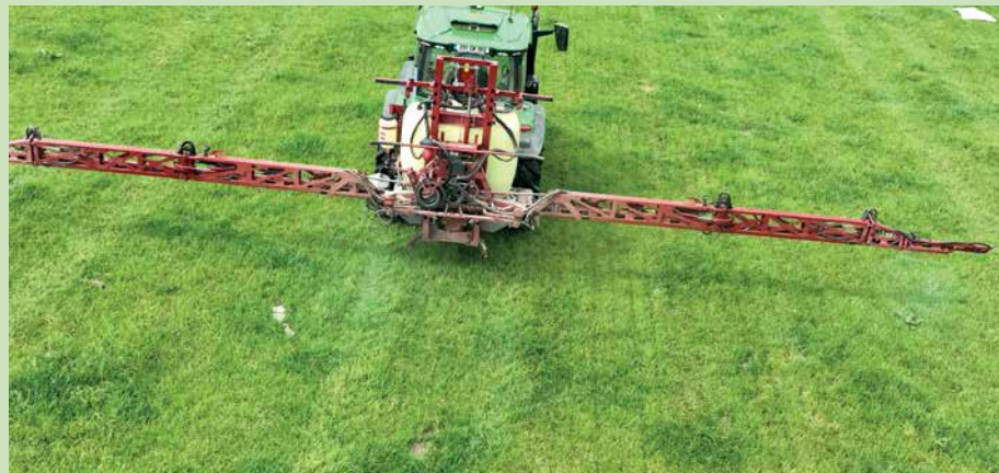
Syngenta optical spot spraying trials to target grass weeds in pasture - Ireland 2023
