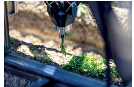
The Weader can identify and precisely remove weeds within the crop rows.
