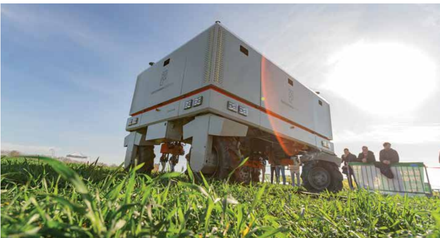
Hoes on the Robot One's controllable arms can be substituted for a streamer, rotor harrow, L-Bow or even lasers.
