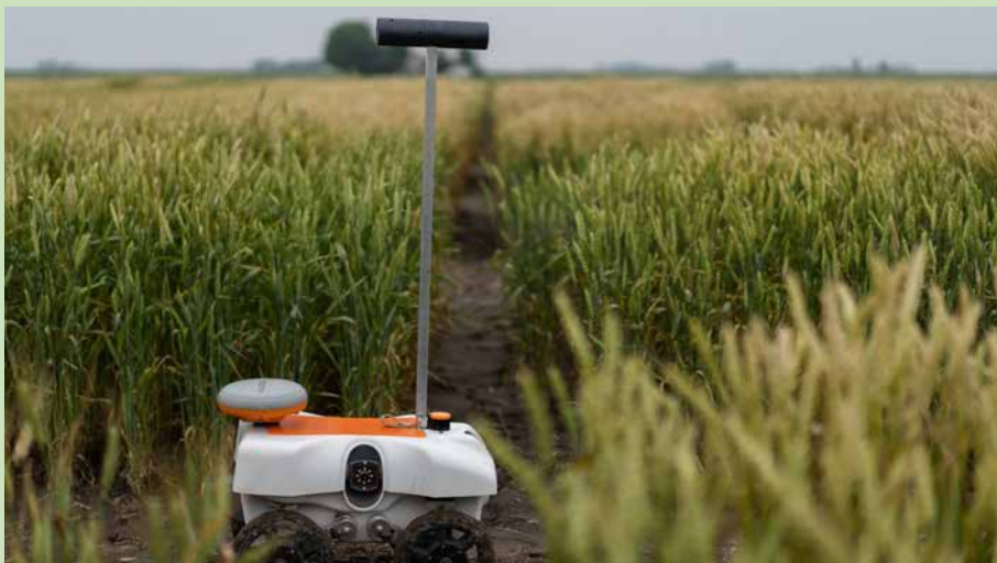
KWS is using the TerraSentia robot to collect phenotypic data at its trials site in Illinois. PHOTO: KWS.
