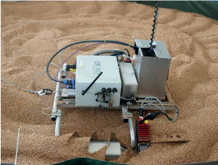
Crover no longer burrows into the heap but crawls along the top on two Archimedes screws.
