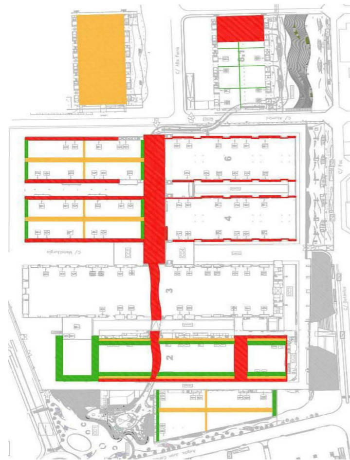
■ Area with special conditions for the placement of the Rigging ■ Area with impossibility to place Rigging ■ Pre-Rigging Area placement of special structure
