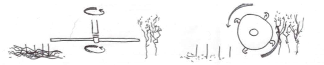
Figure 1: Operation of a Topper (left) and a Mulcher (right)
