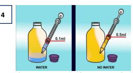
If testing water, draw 0.1 ml from the bottom of the sample using the syringe. If testing fuel, draw 0.5 ml from 3 cm below the sample surface. Both water and fuel can be tested separately if required.
