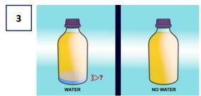
If sufficient free water is present, this should be tested separately from the fuel (recover the water into another smaller container if needed). If no water is present, the fuel must be tested.
