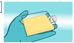
Tap the test firmly in the palm of your hand until the gel forms a flat layer on one of the bottle's larger flat sides.
