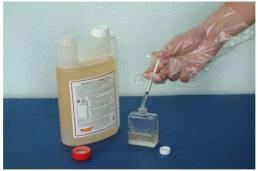
1. Break and discard the plastic seal. Remove the bottle cap and place on a clean surface with the inside face upwards. Use the syringe to add 0.5 ml fuel or 0.1 ml water to the MicrobMonitor2 bottle. Recap and label the bottle.
