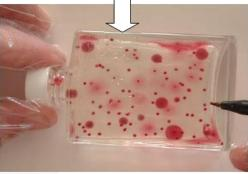
6. To examine test, hold bottle against a light background and count all of the red / purple colonies, marking them off on the bottle with a felt tip pen. Re-incubate and examine if necessary for up to 4 days (see Notes). If numbers are high an estimate can be made by comparison to the chart provided. Record all results and sample information.
