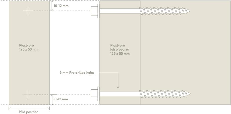
NOTE: Screw fixing method using Durafix hex head screws is for braces or noggins. If a joist is to be fixed then the use of truss clips with screws is recommended
