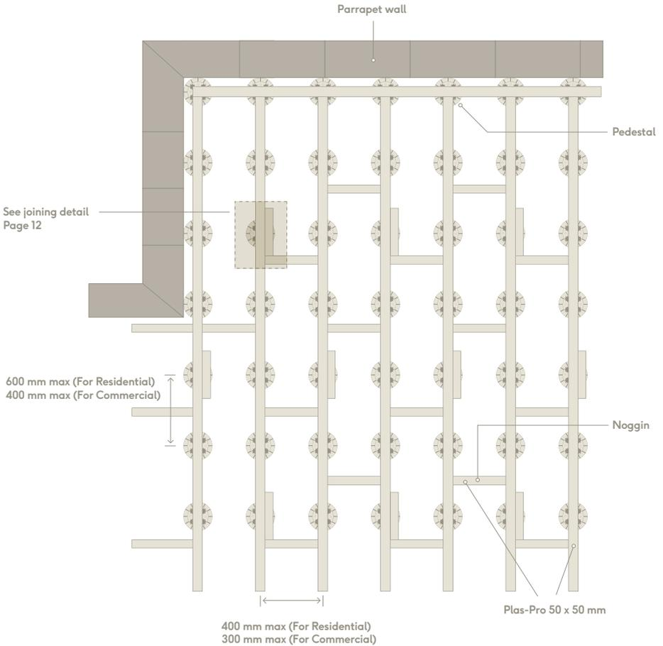
Roof terrace standard subframe laying pattern
