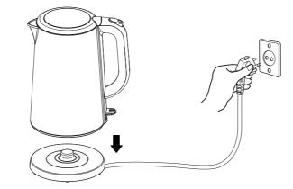
**3**.Close the lid and place the kettle on the base, pluging in the socket.
