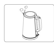
5.The on switch will "click", switching off automatically when water gets boiled. The indicator light goes out at the same time
