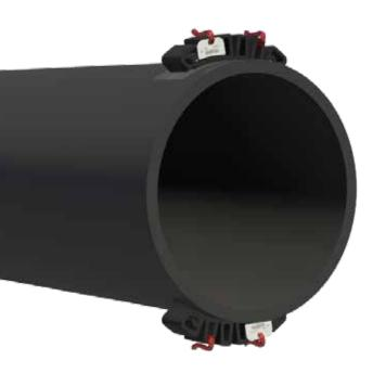
The restraint is a flexible bar, which is fused to the pipe by electrofusion to create a welded shoulder that can restrain the axial movement of pipes in various applications:
