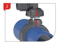
Saddle body is positioned in place and connected to the clamps by hand tightening of the retaining nut. No small parts (nuts, bolts) that may fall and disapear in the trench are involved.
