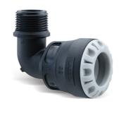
Plasson's Series 1 push fit compression fittings allow for a simple, time effective connection of pipes in diameters 20 to 63mm. fully pressurised leak free water (up to PN16) or air (up to PN10) systems. Ideal solution for connection of airing systems and small diameter water lines. Available in wide range of geometries.
