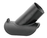
Saddles with 110mm 45° inlet, weldable to thin walled pipe mains, SDR11 to SDR26, covering diameter range 160mm to 315mm
