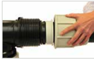
Insert the pipe into the body of the fitting until it meets the interior stop. Then draw the 'O' ring and collars close to the body of the fitting.
