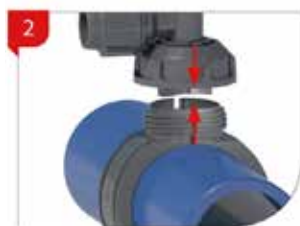
Saddle body is positioned in place and connected to the clamps by hand tightening of the retaining nut. No small parts (nuts, bolts) that may fall and disappear in the trench are involved.
