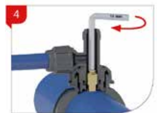
Tapping of either live or unpressurised PE and PVC pipe mains is achieved by operating the integral cutter with a 12mm hex drive.
