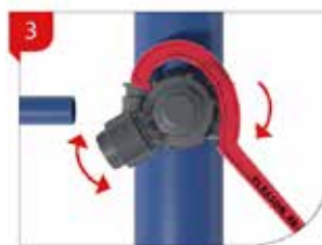
Use PLASSON mechanical spanner to rotate the nut another 1/2 turn and firmly secure the saddle in place. The outlet is then rotated and secured in the desired direction by tightening the grey nut.
