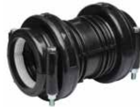
Open the white split ring and mount onto pipe with larger side against the collar ensuring that both parts meet the body of the fitting. Screw the nut tightly onto the fitting using a PLASSON wrench.
