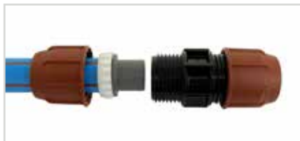
Push the barbed end of the adaptor into the pipe until it meets the stop (a mallet may be required). Then push the plain end of the adaptor into the fitting until it meets the stop.
