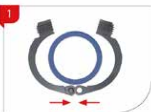
The two clamps of the saddle wrap around the pipe and snap together. The saddle is now retained on the pipe and the installer is free to keep working.
