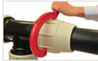
Tighten the nut with a PLASSON wrench until the 'O' ring and collars enter the fitting and reach their end position. Unscrew nut from fitting.
