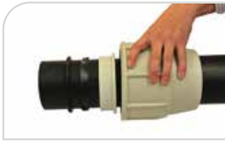
Draw the nut, collars, and 'O' ring over the end of the pipe to a distance of approx. 250mm (put the white split ring to one side for later use).
