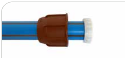
Remove nut and grip ring from fitting and mount brown nut onto the pipe and assemble grip ring flush with the pipe end.
