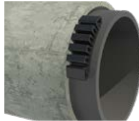
Blocking pipe movement after slip-lining.
