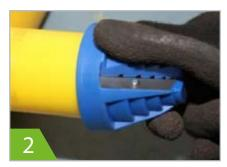
Ensure the spigot or pipe end is clean and free from surface scratches or damage. When using 63mm pipe, use the Plasson chamfer tool for ease of insertion.
