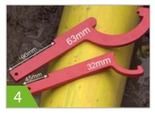
Using the depth gauge on the PLASSON wrench, mark the spigot/pipe end. This shows the minimum depth required. The main body has a center stop so it cannot be over inserted.
