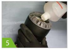
Apply a leak detection fluid directly onto the sealing ring, as lubrication will ease the insertion.
