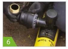
Loosen the locking nut two or three turns, then slide onto the spigot/pipe. Once you have reached the center stop, or passed the minimum depth marker, re tighten the locking nut until the mark on the locking nut meets the mark on the main body.
