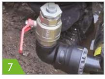
Once the application has been completed and the fitting is no longer required on the spigot/pipe, loosen the locking nut sufficiently and slide off. Retighten and store for the next use.
