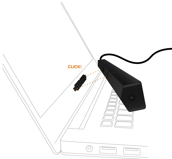
Figure 8. Place the mounting bracket on the bezel so that the Pro Fusion is as close to the bottom of the screen as possible without covering the screen.
