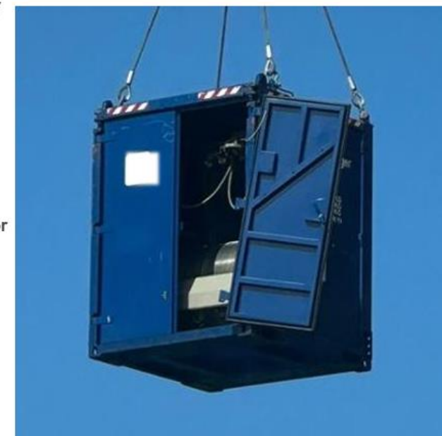
Locking device locks in the middle of the frame only, not to the top and bottom as required by the design standard
