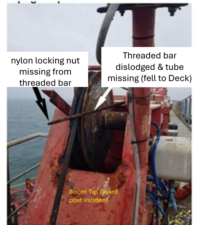
Rope Guard Tube Missing
