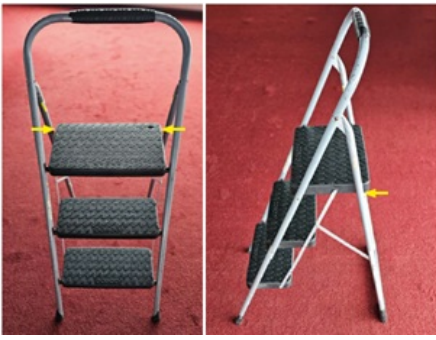
Stepladder, showing the location of the failed metal support
