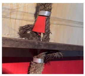
A number of incidents / safety concerns / observations have been reported recently indicating an increasing trend of vessels presenting unsafe pilot boarding arrangements which do not meet the requirements set out in The International Convention for Safety of Life at Sea (SOLAS) Regulation V / 23 and IMO Resolution A. 1045(27) (as amended).
