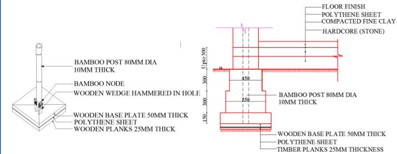
Foundation Details of Strip Footing Masonry Foundation and DPC (Where cement and concrete not available)
