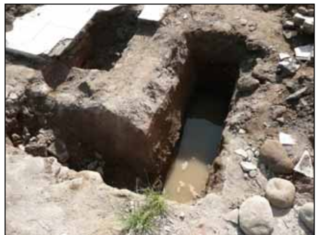
Soil tests: water saturated down to ~1 m (vicinity of rice fields)
