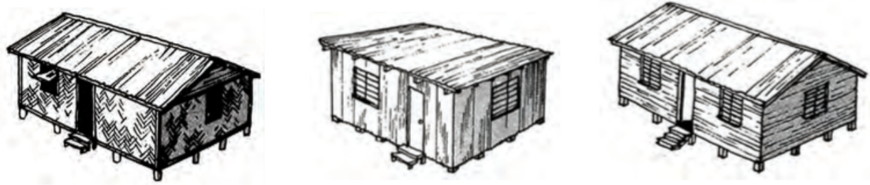
Wall types of transitional timber-framed housing (from left to right): with woven mats, CI sheets and timber boards (©Interact)
