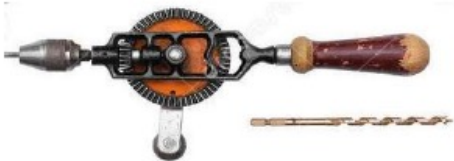
Manual drill: "Berbequim" with bits (1mm, 3mm, 5mm)
