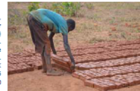
Bricks are hand moulded in wooden moulds. Brick production in Benga, Mchinji. © Jon Twingi.
