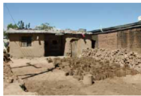
Production of adobe bricks in a peri-urban area near Blantyre. © Carmichael C.
