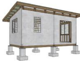
12 PHASE 2 - FIBER CEMENT WALL PANELING OPTION SCALE: 1/8"
