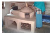
Energy efficient stove made of chikko in the village of Awra Amba (Amhara). It improves the quality of the air inside the house. © Laurence Fontana
