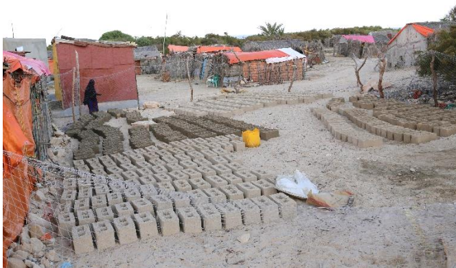
Production of cement hollow blocks in Puntland (CC – Heimo Liendl)
