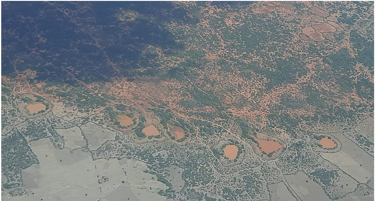
Surface water collection and storage systems are very common in parts of the country. Wars (open air water reservoirs) close to Baidoa CC – Enrique Sevillano Gutiérrez – CRAterre
