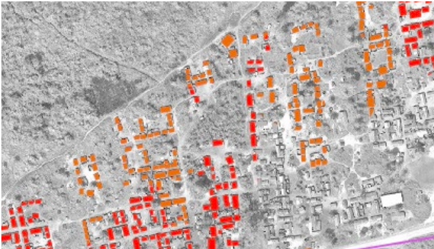
Snapshot of the flood risk map of Bétou settlement: the colour depicts the risk level for each building (orange = medium, red = high) © N.Antenen, ETHZ
