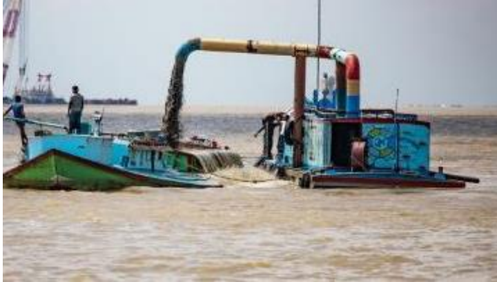
Sand collected from nearby river for block manufacturing
