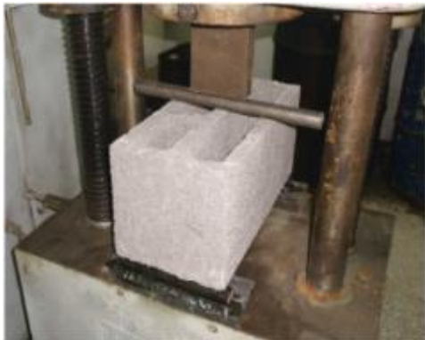
Block strength tested in HBRI lab.
