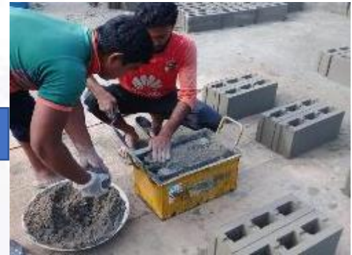
Mortars are fed into dies to produce blocks
