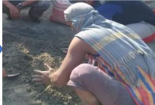
Sand, cement and chemical (ASTM C-494) mixing by hand for block manufacturing
