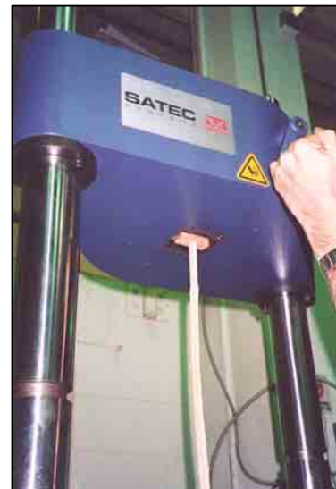
Fig 14.2: Specimen loaded in tester
