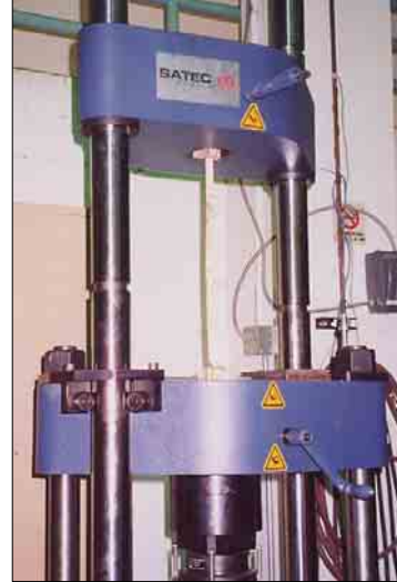
Fig 14.3: Glued specimen loaded for testing
