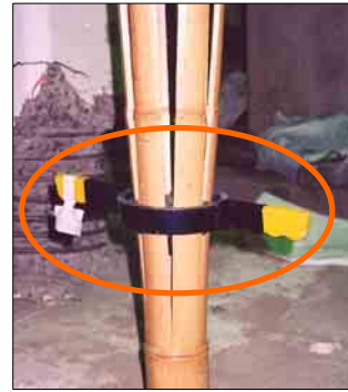
Fig 15.7: Bamboo Splitting method
