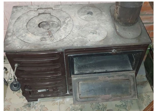
Figure 2. Thick-walled stoves for fuel with high heat capacity.
