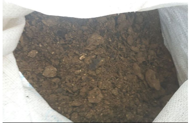
Figure 5. Briquettes damaged during unloading.
