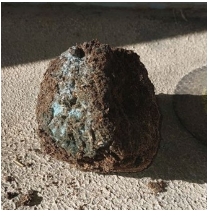
Figure 6. Wetting of briquettes due to improper storage.
